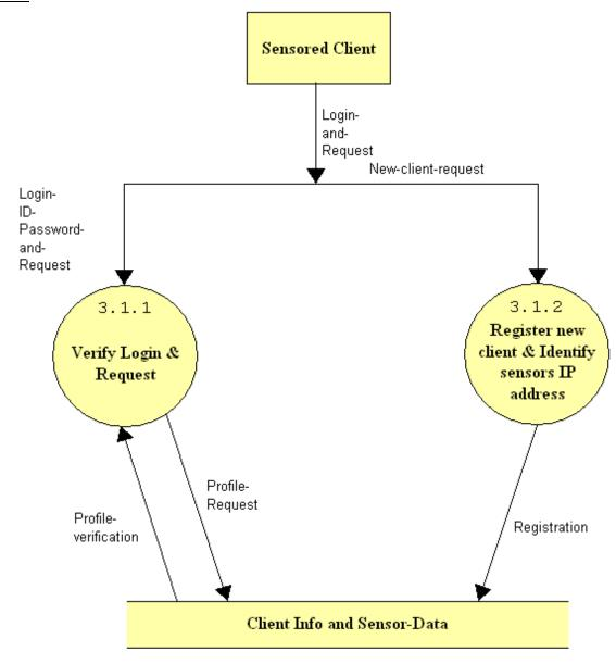
This shows the process for the "Verify Login and Process Request" method.
