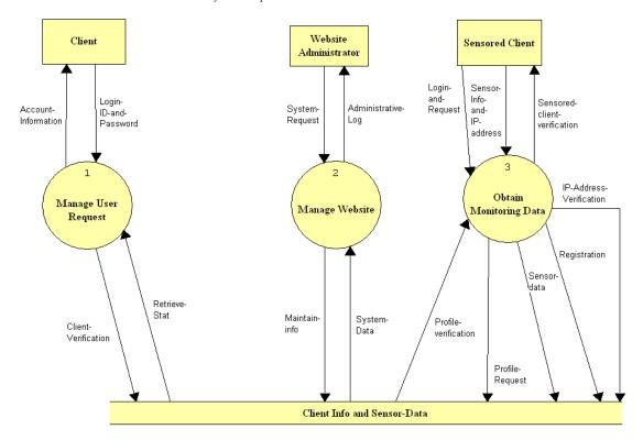
This is the level 0 diagram. This diagram is an expansion of the "Environmental Monitoring System" process from the context diagram.
