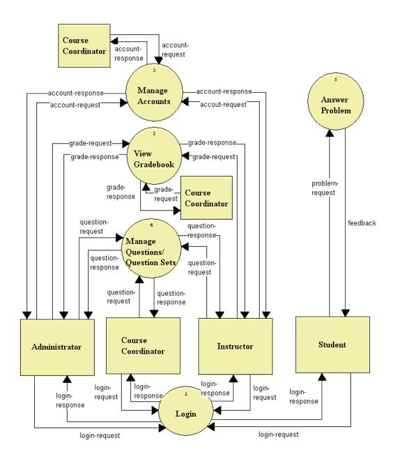
The Level 0 diagram is an expansion of the Javanet System process from the Context Diagram. It outlines all the major processes of the system and how they interact with each of the users.
