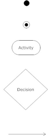
**Initial Node -** The initial node is the first node in the process. The initial node is the starting point for all movement.
