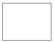
System Boundary- Represents the limitations of the system. All processes of the system are contained within the system boundary. All outside entities are represented outside the system boundary.
